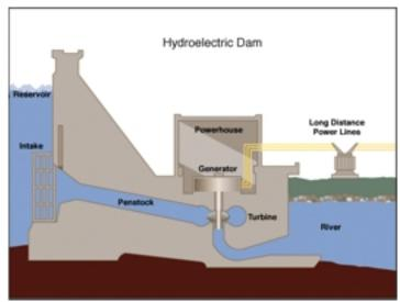
In either instance, the water flows through a pipe, or *penstock*, then pushes against and turns blades in a turbine to spin a generator to produce electricity. In a
